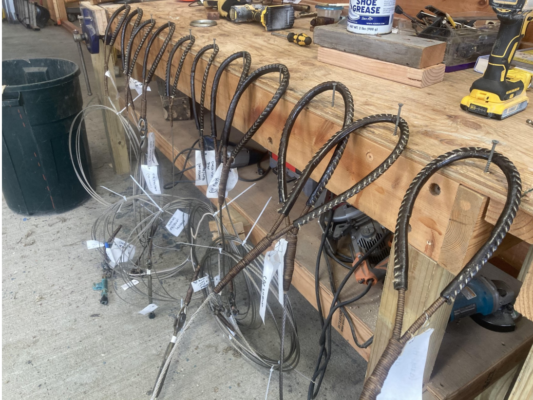
Clara J's Standing Rigging re-Served and ready for spring.
